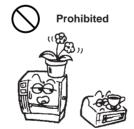
■ Do not place metal objects or water-filled containers such as flower vases, flower pots or mugs, etc. on top of the machines. If metal objects or spilled liquid enter the machines, this may cause **fire** or **electric shock**.
